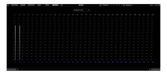
The 'Meters' tab provides up to 32 individual peak meters for each row from '6.4.1.
