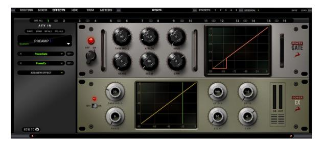
The 'Effects' tab lets you apply up to 8 FPGA FX per mono audio channel for a total of 16 channel strips and 128 FX instances, independent of sample rate. However, different types of FX place different processing loads, resulting in the following instance limitations:
