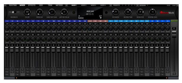
The Mixer tab is home to four 32-channel virtual mixers. Each channel is equipped with Pan, Volume, Solo, and Link controls (on odd-numbered channels), as well as metering. The Master channel has Volume and Mute controls.
