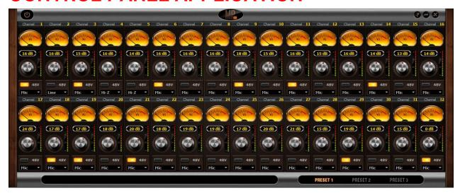
The MP32 Control Panel application lets you control all the functionality of its hardware. There are two different types of preamp section on the MP32 control panel, one which is HiZ enabled to the first four preamps and the rest of the preamps which control only mic/line levels.
