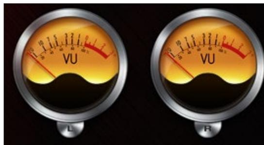
Virtual volume meters for the L/R analog and monitor outputs.
