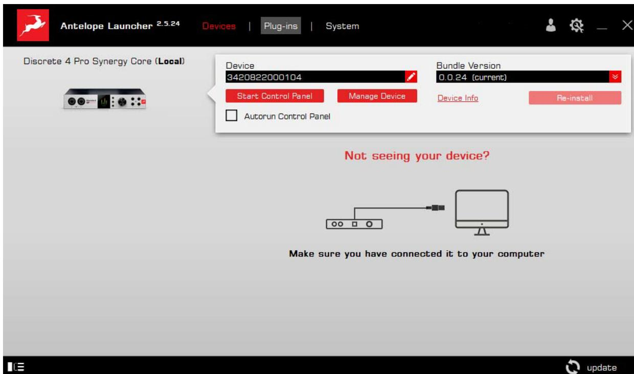
All Antelope Audio devices currently connected to your computer are listed in this section. In this example, we have connected the Discrete 4 Pro Synergy Core. However, the application functionality is identical for each Antelope device.
