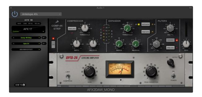
Available as a separate purchase, AFX2DAW is a bridge plug-in for using Synergy Core FX as inserts in your DAW. All Synergy Core FX processing and I/O audio streaming activity is
