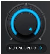
Retune Speed controls how rapidly the pitch correction is applied to the incoming audio. The units are milliseconds. A zero setting will cause immediate changes from one pitch to another and will completely suppress any vibrato or deviations in pitch.
