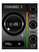
This is a single mic/combo input with a gain adjustment knob, peak metering and controls. There are 12 such inputs in the Orion Studio Synergy Core Control Panel. Inputs 5 to 12 have built-in mic emulations.
