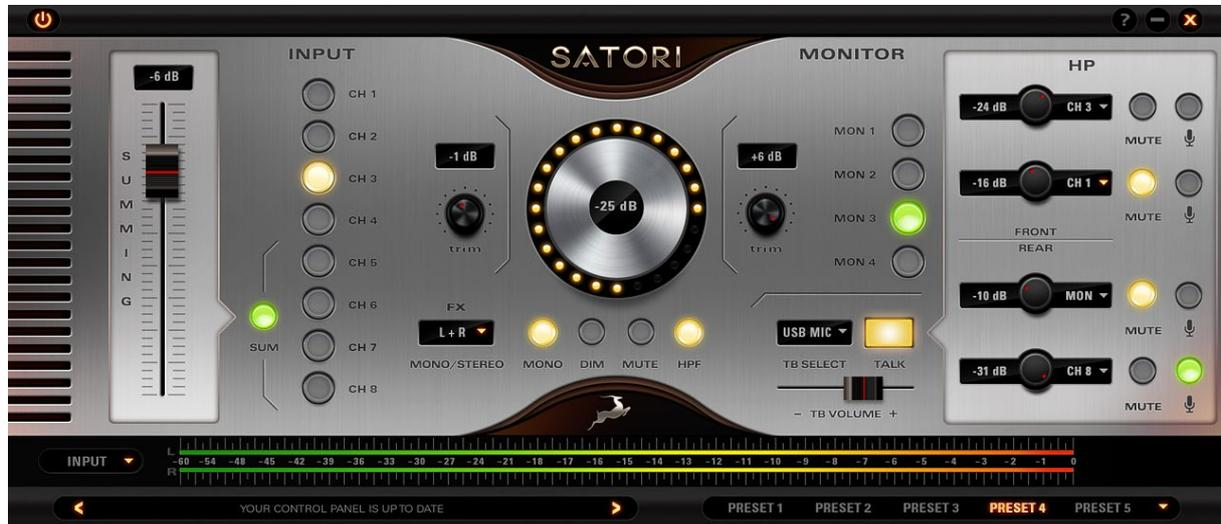
The Windows & macOS Control Panel application mirrors the functionality of Satori's front panel controls, not unlike how R4S does it. It also provides metering and save/recall of up to 5 presets. Click on PRESET 1 - 5 to recall a preset. Ctrl + Click (Win) / Command + Click (Mac) on PRESET 1 - 5 to save into that slot.
